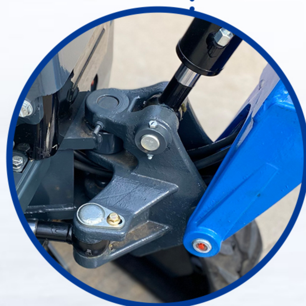
Integrated Casting of Boom Bracket
