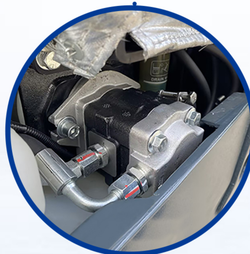
3 pumps combined configuration
