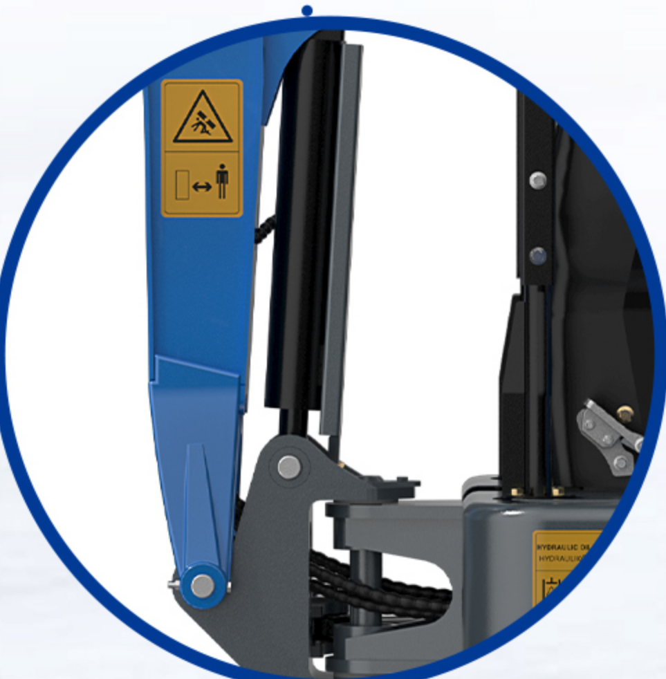
Top-mounted boom cylinder + cylinder guard plate
