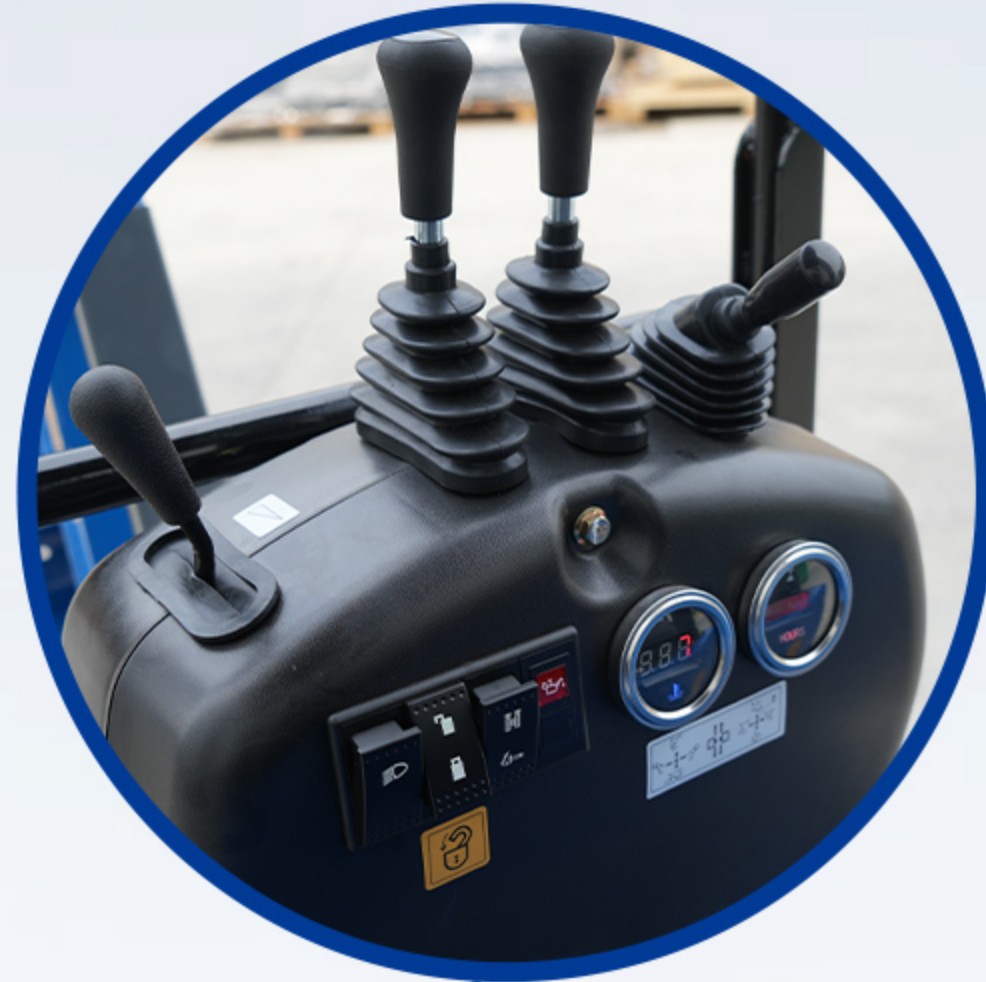
Operator protection hydraulic lock
